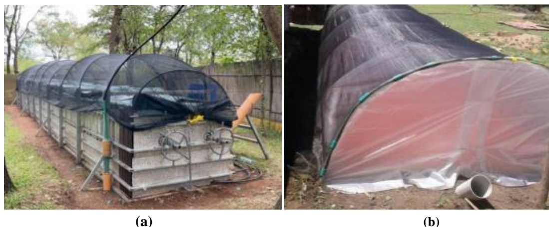
Figure 1: a and b: C25 Medium (Medium commercial biogas digester) and D9 Digester (Domestic biogas digester): Source – Verde Technology 2019 Annual Report.
