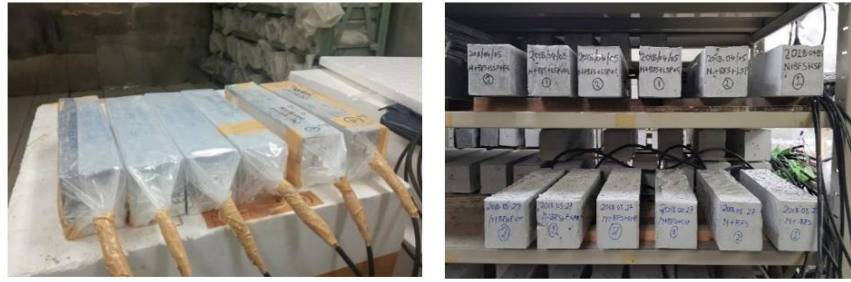
Figure 3: Shrinkage measurement for Autogenous (Left hand side) and Drying Shrinkage (Right hand side)
