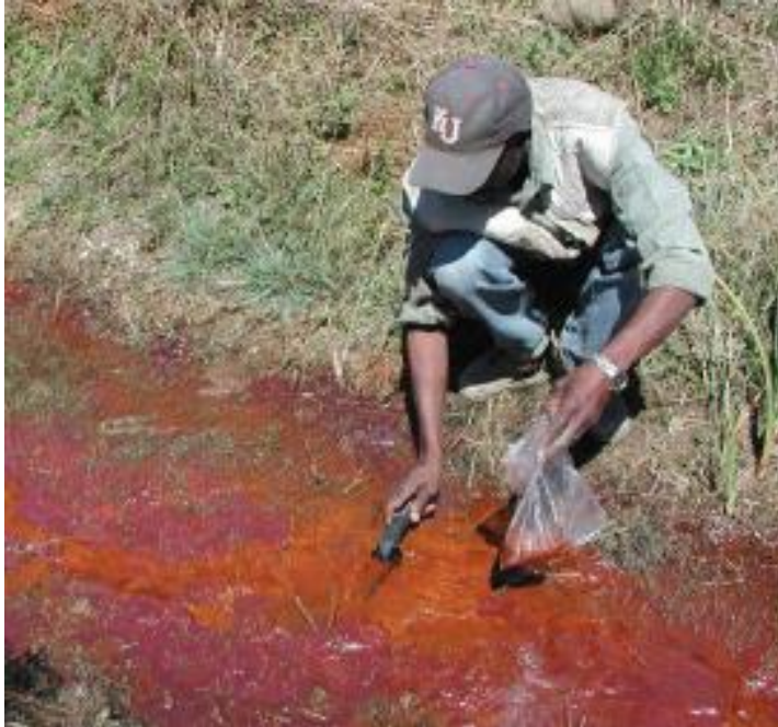
Toxic sludge seeping from the Muntimpa tailing dam into the environment.
