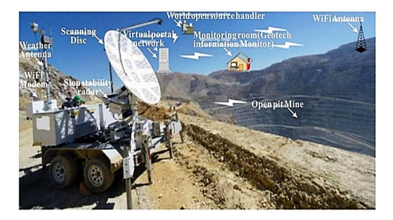
Figure 1 :Slope stability radar field deployment at Nchanga open pit (KCM, 2014)
