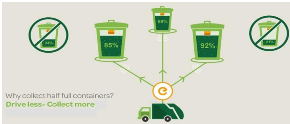
Fig 5: M2M/ IoT can allow the bins to share data they collect to optimize waste collection (Enevo 2014)
