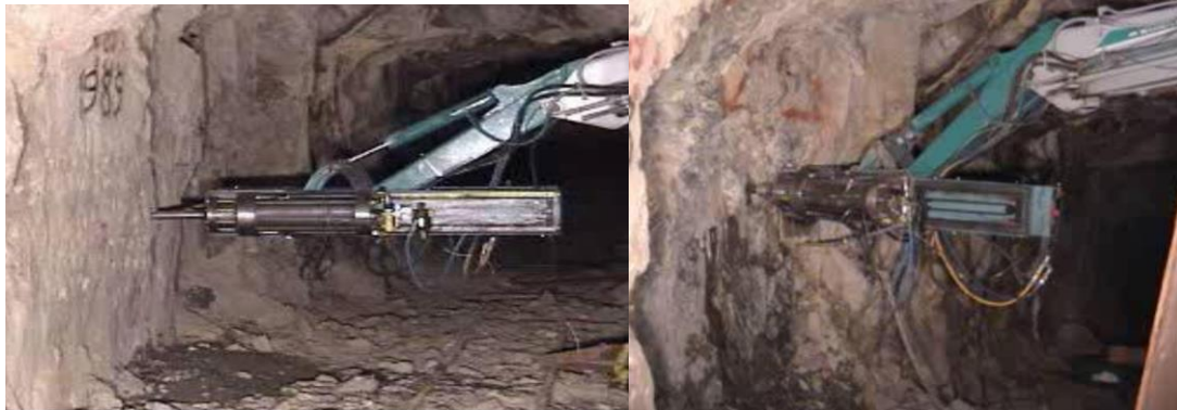
Figure 8. Continuous Mining – Control Foam Injection (Pickering and Young, 2016)
