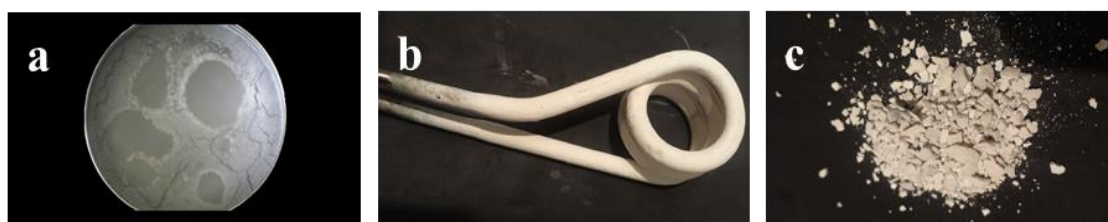
Fig. 1: (a) precipitate in boiling water; (b) precipitate scale on the heating element; (c) scraped precipitate from a heat exchanger surface
