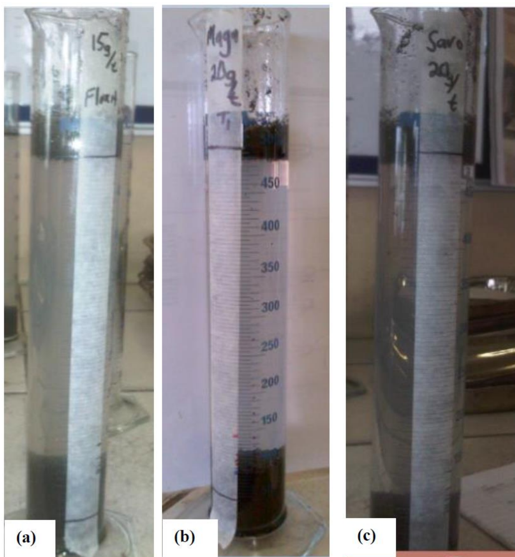
Figure 6: Clarity profiles of the supernatant liquid at the Optimum settling dosages. (a) 15g/t of Floxit, (b) 20g/t of Magnafloc and (c) 15g/t of Savofloc
