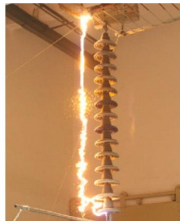
Figure 4: Birds droppings creating a short circuit on the transmission network (Source: Rens, 2022).
