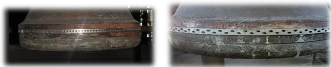
Figure 6: Original and modified distributor plates
